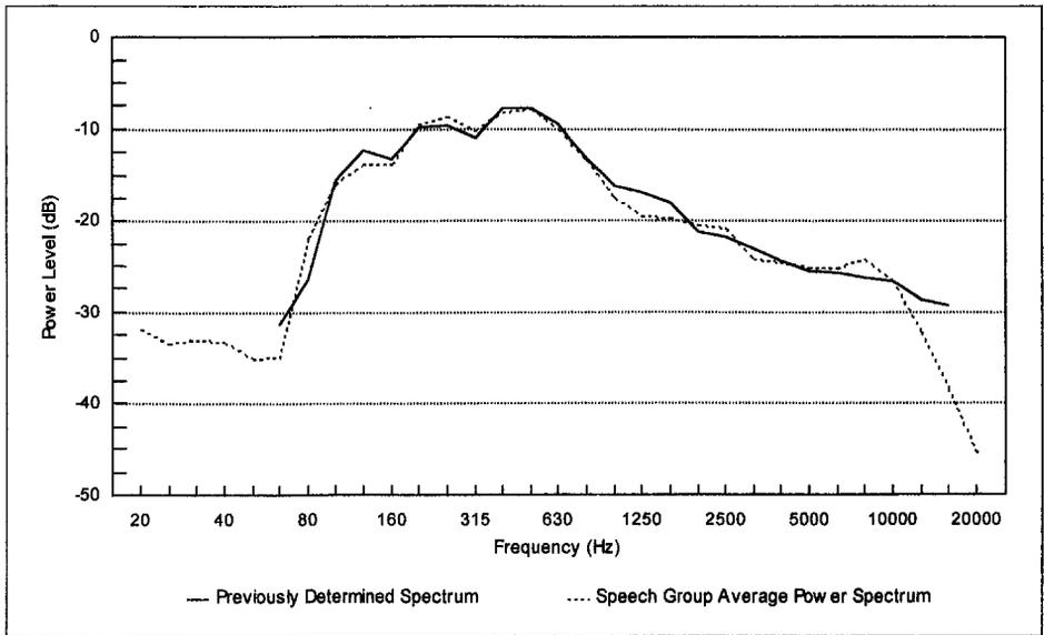
**Figure 2** Comparison of newly measured speech spectrum with previously determined spectrum.
