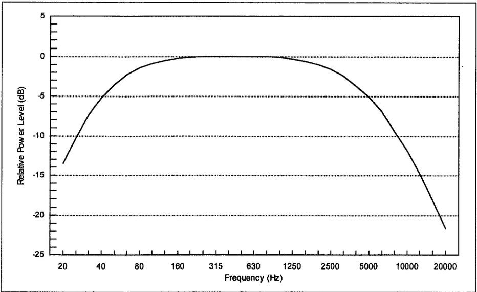
**Figure 1** Average Power Spectrum of IEC 268-1 Simulated Programme Signal.
