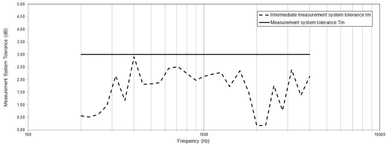
Figure 14 Measurement tolerances calculated from the 30 MSA measurements in figure 13
